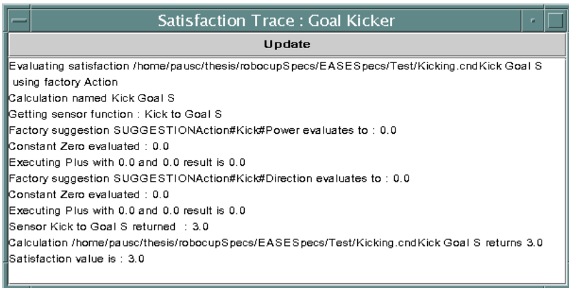
Fig. 5. The Calculation Trace window shows the details of the calculations one of the agents is performing. Each line shows the result of computing the value of one cell. The labels of the cells are printed with the corresponding intermediate results. The bottom line in the window shows that the final satisfaction value calculated is 3.0.
